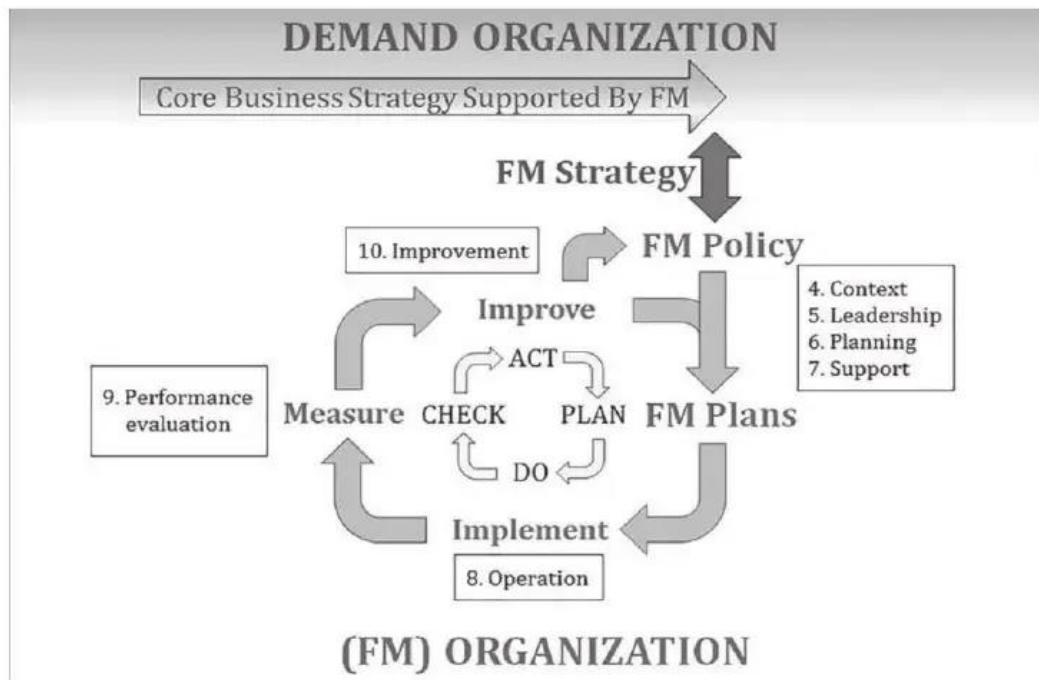
Figure 1 —process approach methodology in facility management
